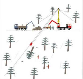
Operation procedure downhill with Mounty-U: The radio-controlled LIFTLINER carriage is operated in a haulback system. Thanks to the integrated hoist winch, the carriage can be moved on the cable and pulling the load at the same time (safe, controlled travel with the carriage to protect the tree population)
